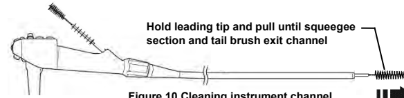
Figure 10 Cleaning instrument channel
